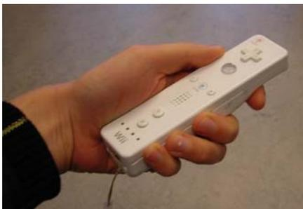
With this setup we are able, in real-time, to steer the tool mounted on the robot just by moving and tilting the motion sensitive Wiimote. This turns the Wiimote into an extremely intuitive input device because the robot is effectively matching the position and orientation of the Wiimote in the hand of the user.
