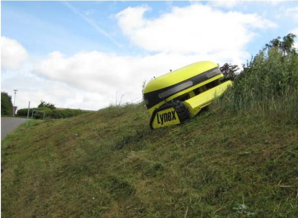
CASMOBOT is able to determine its current position and attitude using a high accuracy RTK GPS system and attitude sensors. An advanced dynamical route planning algorithm running on a small linux computer will ensure that the grass is cut at all parts of the area. Even at high slopes the CASMOBOT will do the job crunching through the high grass.
