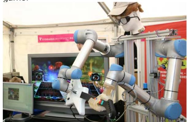
The hand, designed by Thomas Priisholm who has recently graduated as mechatronics engineer from SDU in Sønderborg, is actuated by five small pneumatic cylinders and was designed specifically for the guitar. To make the hand look as human as possible and still be able to press all five buttons on neck of the guitar joystick, Thomas took a little inspiration from guitar
