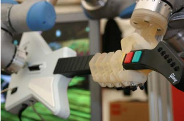
To make the robot actually play the game, a PC with a cheap TV-tuner card was connected to the video output of the Xbox. The open source computer vision software OpenCV was then used to analyze the video signal and calculate when to press the buttons on the guitar with the 5-fingered hand.
