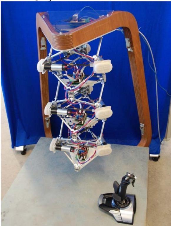
The latest is a complete redesign of the onboard electronics, with the major selling point being that the previous inflexible, monolithic controller has been replaced with a new distributed system. Even though the monolithic controller worked, it required the three sections of the robot to be connected through large, bulky, noise-susceptible ribbon cables, and if something was to be
